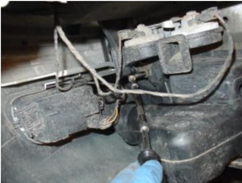
At this point you can clean the alternator cooling duct.
