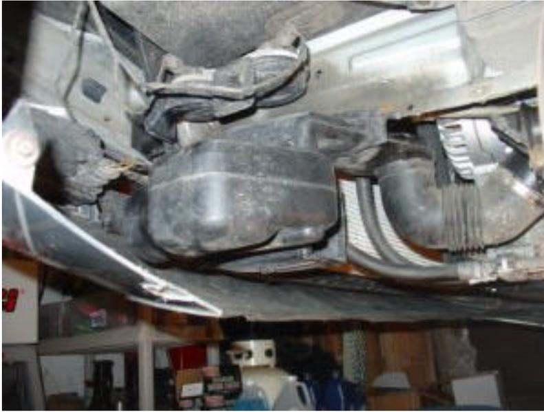
There are three screws holding the alternator cooling duct in place. The forward one is hard to get. I have a universal joint for my 1/4" socket set. It makes this screw much easier to remove. Remove the duct.
