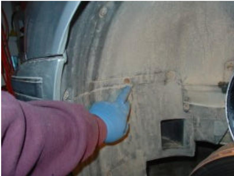
Once the forward-lower fender liner is out, take out the three screws holding the brake cooling duct. Remove the brake cooling duct.
